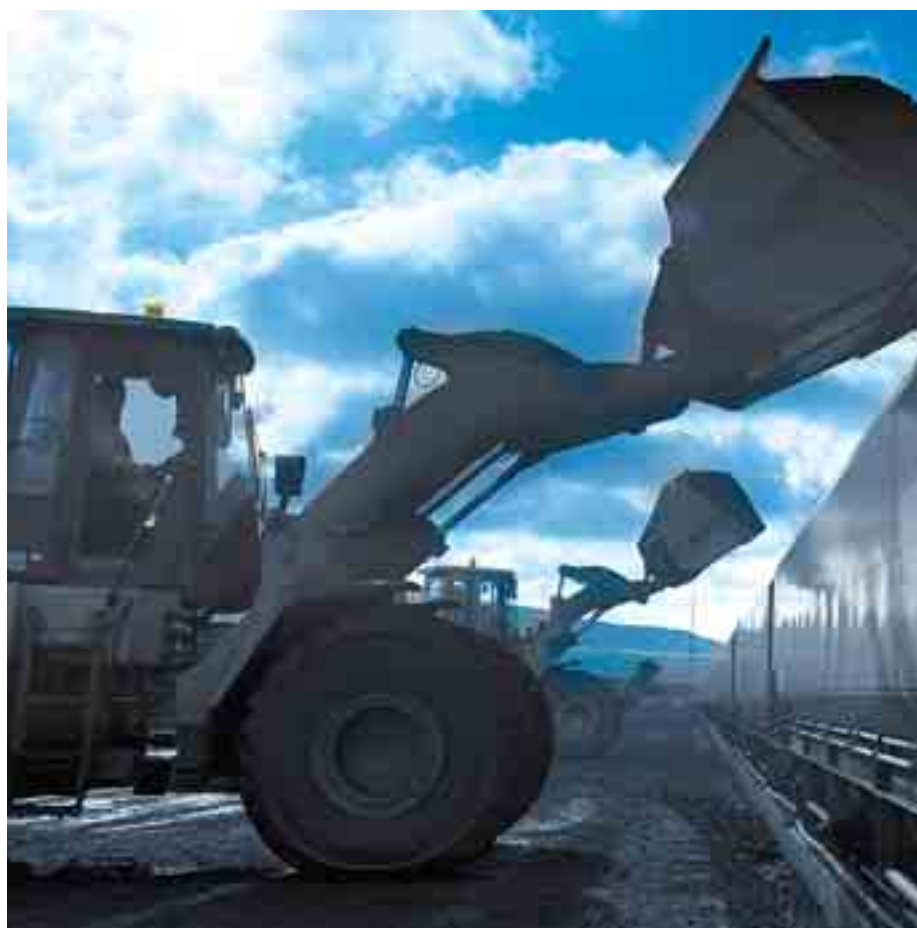
Coal is loaded onto trains at our railhead. Each train can carry 1,400 tonnes of coal in 20 wagons and upwards of 30 trains per week are dispatched.
