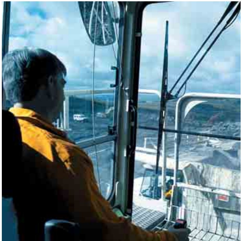
Overburden is removed from above the coal seams by 265 tonne excavators which load 100 tonnes of earth in four passes.
